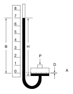
Figure 5-6 Well-type Manometer
