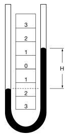
Figure 5-2 U-Tube Manometer Pressure Applied
