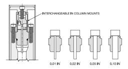
Figure 4-3 Interchangeable Piston & Cylinder Assemblies
