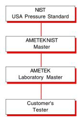
Figure 2-5 Traceability Path AMETEK Deadweight Testers
