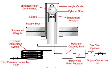
Figure 2-4 Schematic Diagram - Floating Ball-type Deadweight Tester
