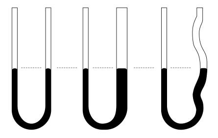
Figure 5-3 U-Tube Manometers Non-uniform Tubes, No Pressure
