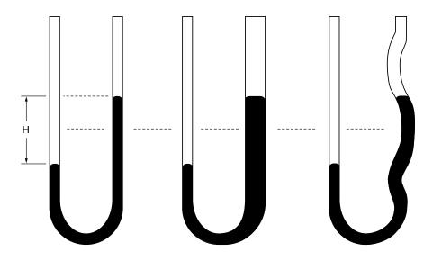
Figure 5-4 U-Tube Manometers Non-uniform Tubes, Pressure Applied
