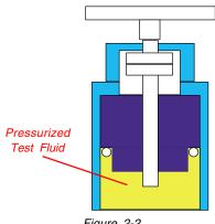
Figure 2-2 Reentrant Type Piston & Cylinder
