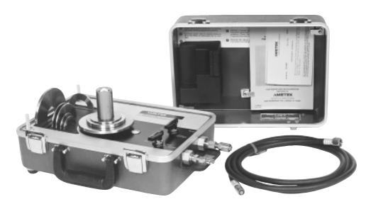
Figure 4-12 Model PK II Medical Pneumatic Deadweight Tester
