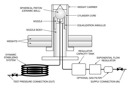
Figure 4-9 Schematic AMETEK Floating Ball Pneumatic Deadweight Testers
