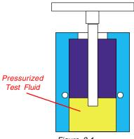
Figure 2-1 Simple Type Piston & Cylinder
