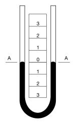
Figure 5-1 U-Tube Manometer Zero Pressure
